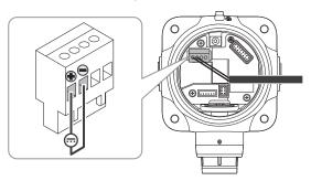
If AC power is used, ensure that terminal 4 "Common" is used to connect the power and controller grounds together.
