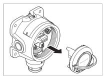
Hold the handle of the main electronics module and pull it outward with a steady force. Do not pull sharply.
