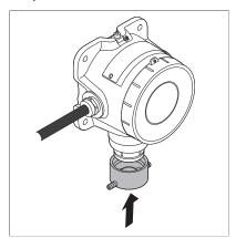
1. Push the calibration cap on the sensor cover as shown.
