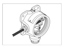
5. Feed the cable through the cable gland.
