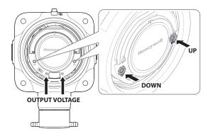
**To inhibit the detector output**: Press and hold the UP button for 2 seconds.
