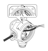
Effective grounding is crucial to ensure stable Modbus communications and to limit the effects of radio frequency interference. A ground point is provided inside the housing. In order to prevent false readings or alarms as a result of ground loops, ensure that the shield of all cables are grounded at a single point, preferably at the controller. Consideration should also be given to how conduit and glands.
