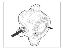
Press and hold the UP button for 10 seconds to switch to sensor replacement mode. In this mode, the detector output is inhibited and the sensor circuits are internally isolated.
