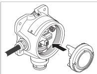
2. Refit the main electronics module to the connector module.
