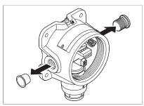
3. Pull out the thread protector from the left cable entry, and remove the blanking plug from the right by turning it counterclockwise. If required, fit the blanking plug to the unused cable entry and tighten it.
