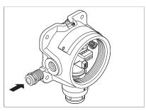
4. Fit suitable cable glands or conduit appropriate to the application and type of cable being utilized to the opened cable entry.
