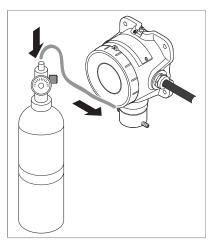
2. Connect a tube from a cylinder of calibration gas to either of the calibration cap's gassing ports.
