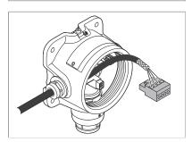
7. Connect cables to the terminal blocks, referring to the relevant wiring diagram. Strip and insert the end of each wire into the corresponding terminal hole. Using a flat-blade terminal screwdriver, tighten the terminal screw until the wire is secured. Use a ferrule on the wire where necessary.
