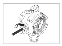
1. Where used, tighten the sealing nut of the cable gland to secure the cable.
